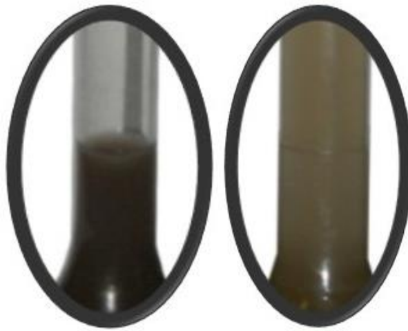
Fig. 4. Comparison of diffusion juice lightness. Left picture: diffusion juice obtained in a conventional diffusion apparatus (RDA at Buinsky Sugar LLC). Right picture: diffusion juice obtained in DPA
