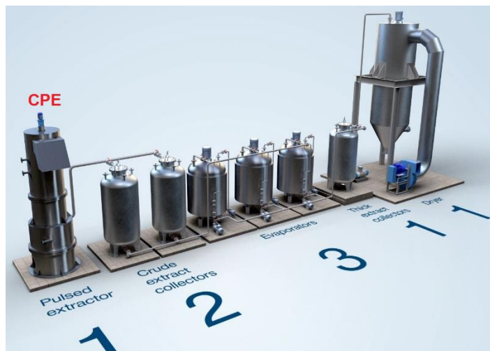
Fig. 6. Comparable throughput line for production of instant chicory powder after modernization to the use of CPE with a feed (roasted chicory) capacity of 400 kg/h
