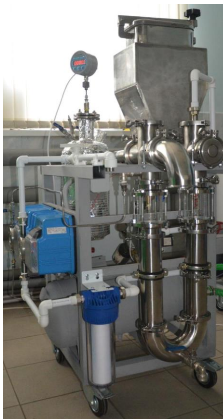
Fig. 3. Pilot pulsating unit (PPU) for extraction
